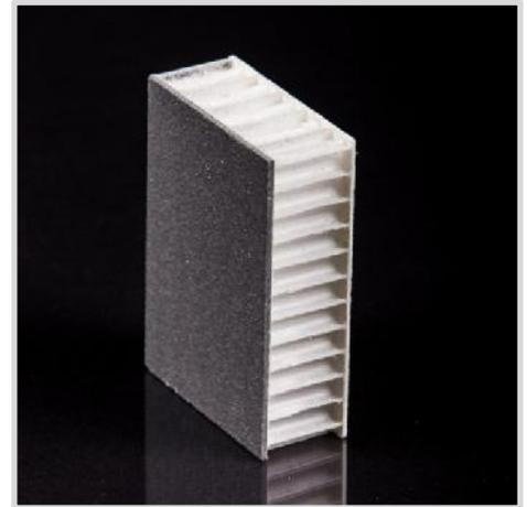
Lightweight panel made of high-strength honeycomb core, a woven glass roving reinforced lower facing sheet as well as a non-slip and wear-resistant GRP top layer.
