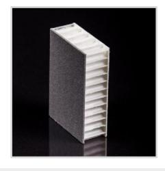
Lightweight panel for truck floor construction made of a high strength honeycomb core, a woven glass roving reinforced lower facing sheet as well as non-slip and wear-resistant GRP top layer.
